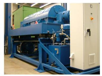
The mud feed pump and the centrate discharge pipe are both fitted with 150mm PN16 flanges.
